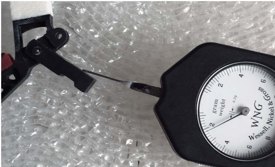
Correct orientation for measuring repetition flange resistance.
