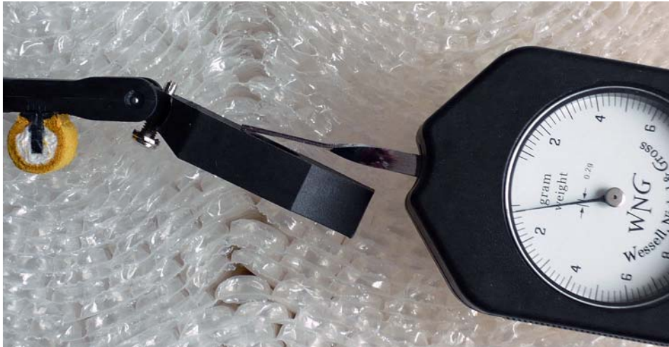
Correct orientation for measuring shank flange resistance.
